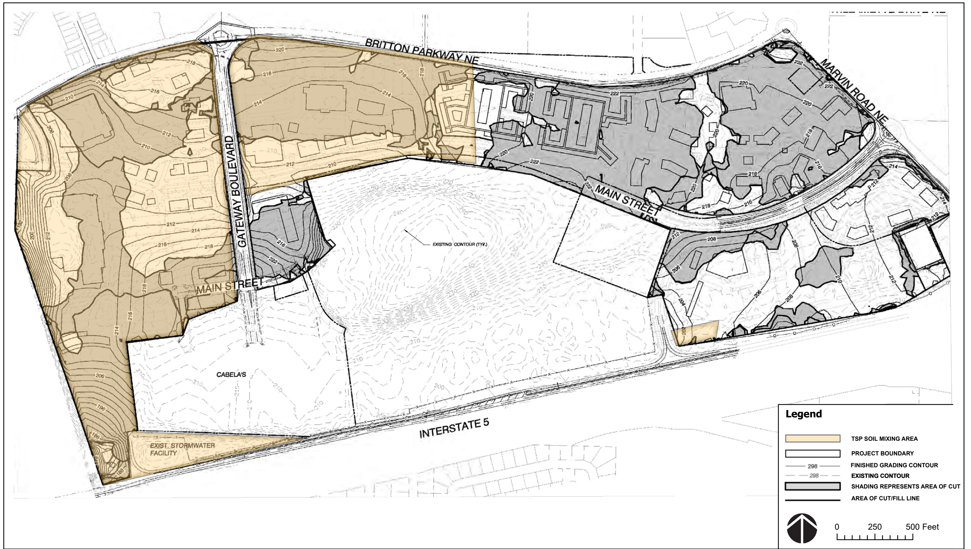
FIGURE 8 ALTERNATIVE 1 - PRELIMINARY GRADING
