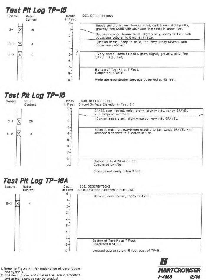
Groundwater conditions, if indicated, are at the time of excavation. Conditions may vary with time. Figure A-8
