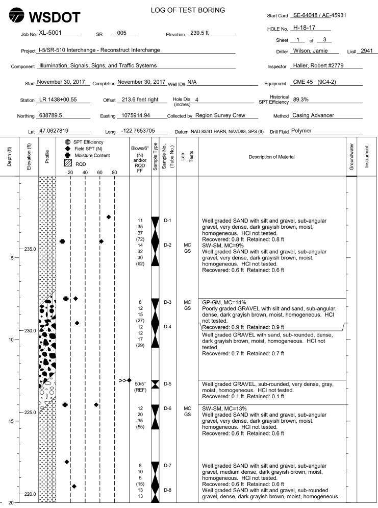
ENTERPRISE BORING LOG XL-5001 005\_510 IC - RECONSTRUCT INTERCHANGE.GPJ ENTERPRISE DATA TEMPLATE.GDT
