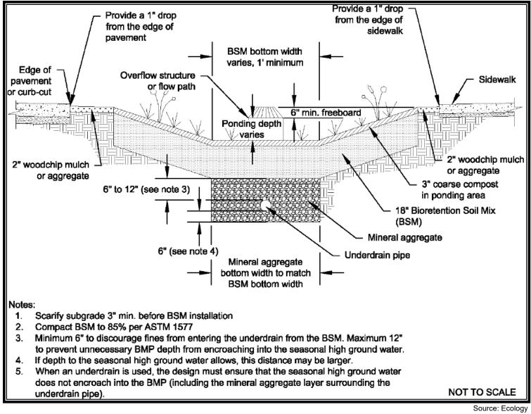
Figure 7.6. Bioretention (shown with optional underdrain).
