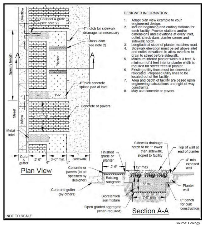
Figure 7.7. Example of a Bioretention Planter.
