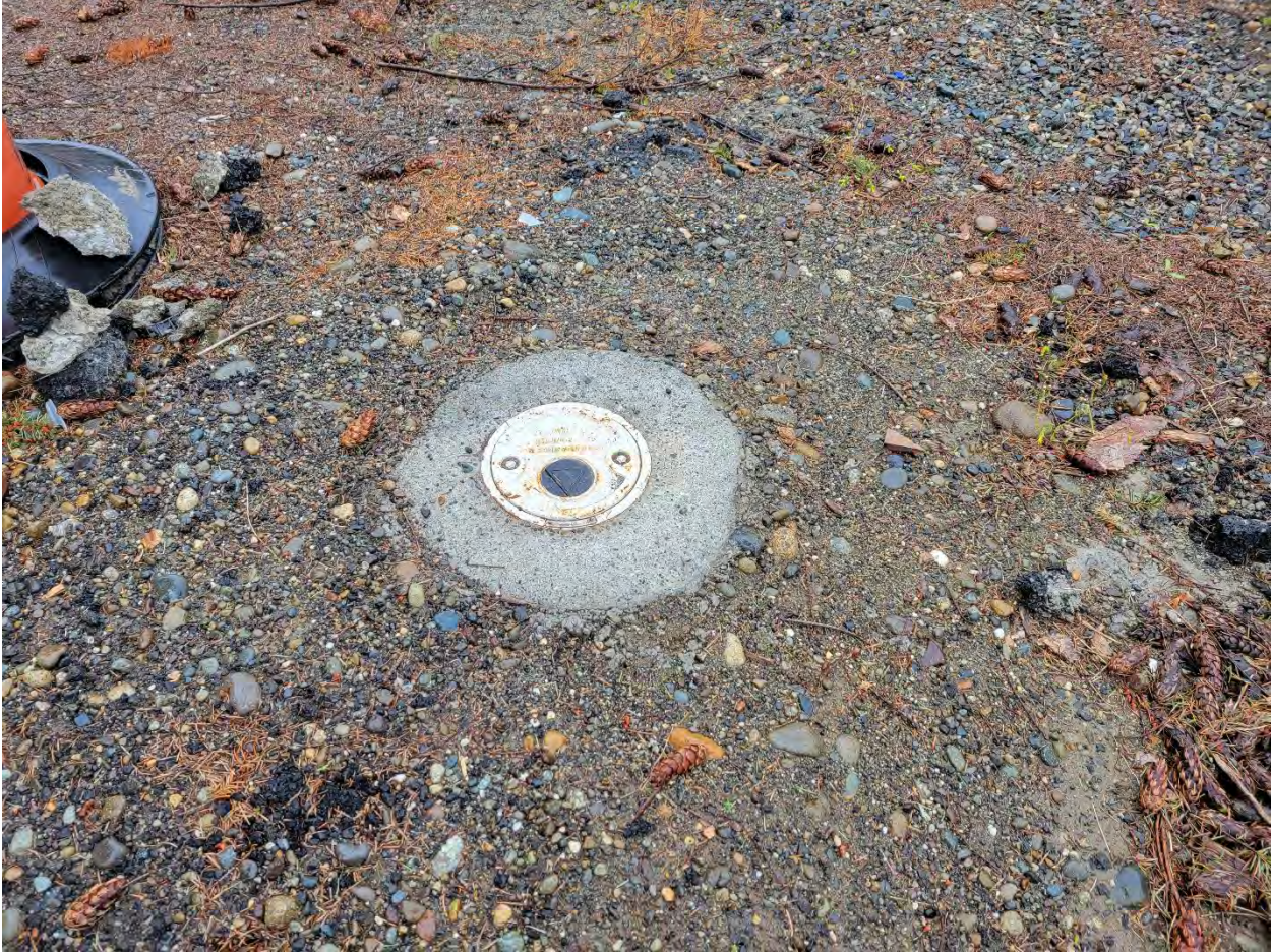
A monitoring well on an off-site property adjacent to Lot 8
