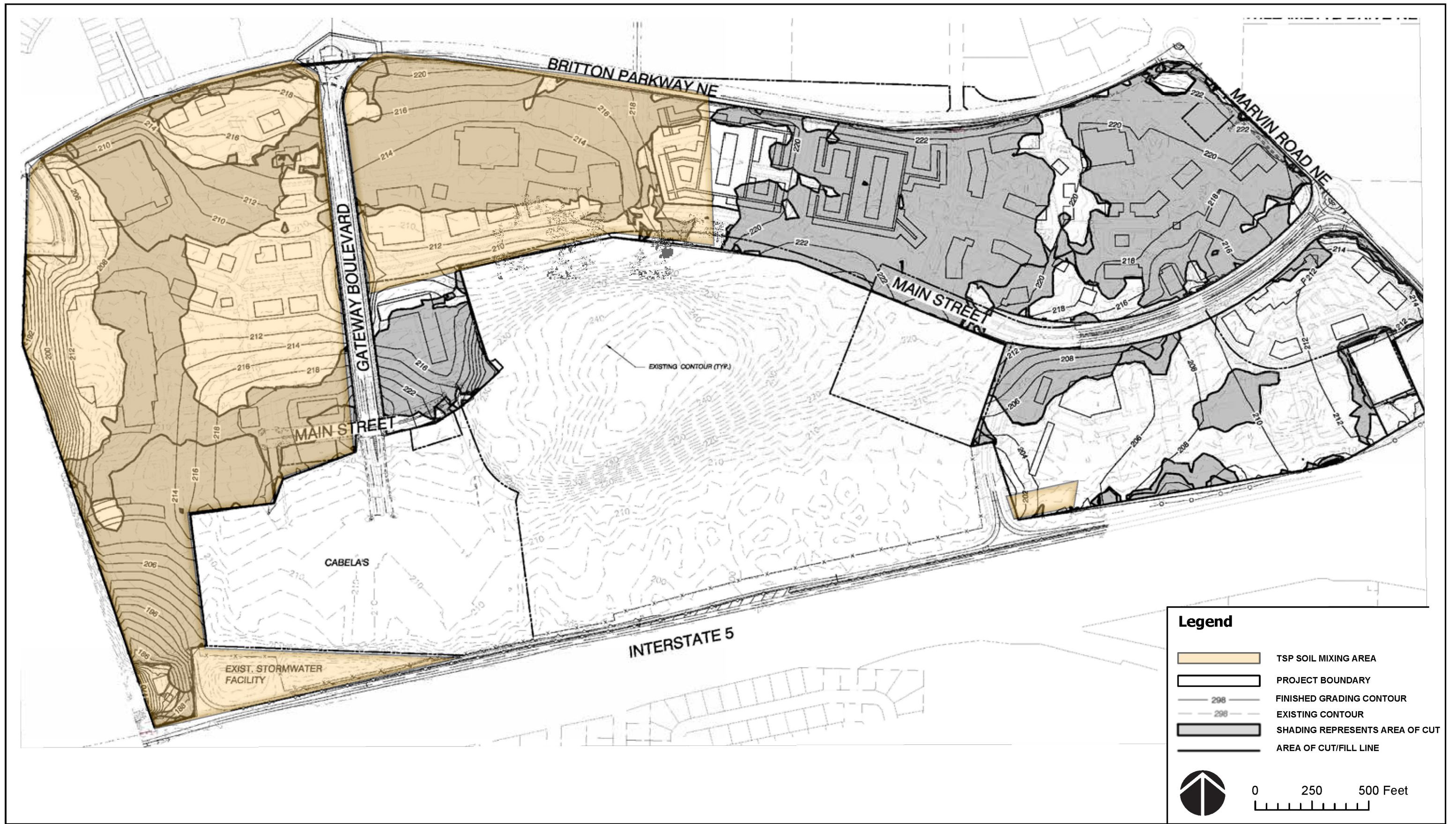
FIGURE 8 ALTERNATIVE 1 - PRELIMINARY GRADING
